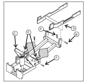
Figure 1. Hitch to Tractor Installation
